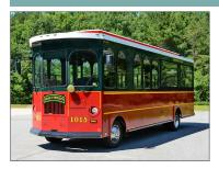
Split passenger cabin with decorative arched sliding vent windows in front and large open window with vinyl roll-up curtains in back.
